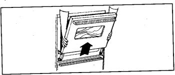
To replace door: Grasp the door at each side, align slots in the door with the hinge arms and slide the door down onto the hinge arms until it is completely seated on hinges.
