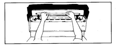
Remove fluorescent tube and replace with an 18 watt fluorescent tube. Snap top trim back into place and reconnect power to range. Reset the clock.
