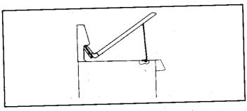
**To lower the top:** Hold the front edge of the cooktop and carefully push back on each support rod to release the notched support. Then gently lower the top into place. The support rods will slide into the range frame.
