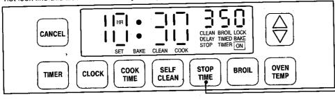
This function pad on your range will be labeled either STOP TIME or OVEN STOP. This pad will operate as described below.
