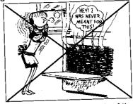
ment. Keep oven vent duct unobstructed. Blockage of the vent prevents proper oven air circulation and will affect oven performance. Avoid touching vent area while oven is on and for several minutes after oven is turned off. Some parts of the vent and surrounding areas may become hot enough to cause burns.
